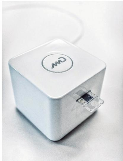
**miDiagnostics' research prototype device that can perform a complete blood cell count from only drops of blood, this prototype device is for research use only, not for in diagnostic procedures**
