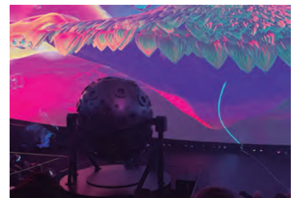
A Zeiss Universarium Model IX projects a realistic night sky onto the museum's Science Dome
